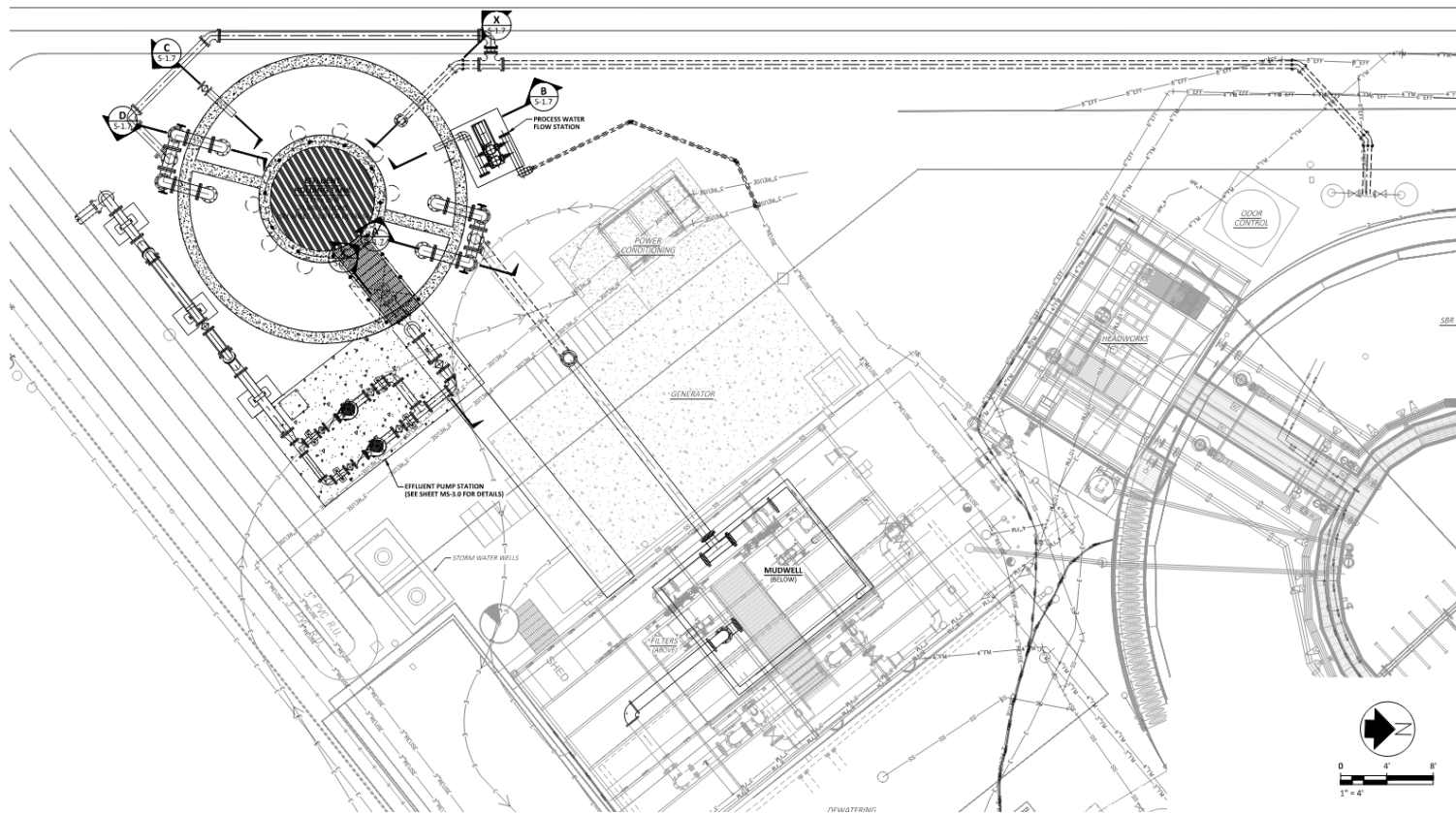
Figure 11. Area 7 WWTP Proposed Site Plan
