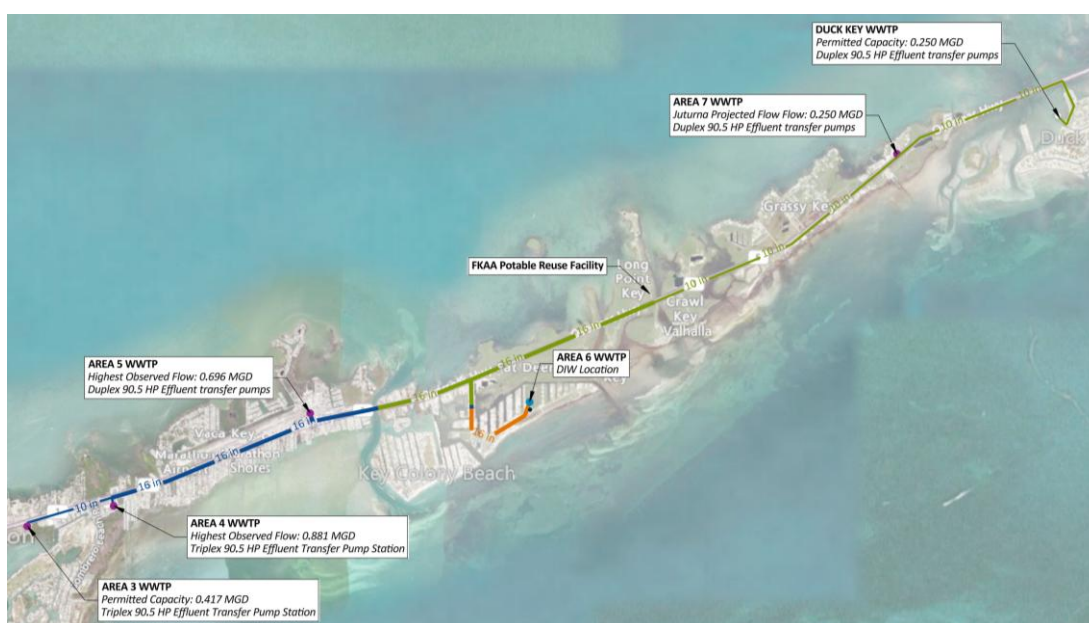
Figure 3. Selected Force Main Diameters and Standardized Pump Sizes
