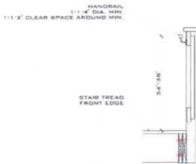
TYPICAL WOOD RAILING ALONG STAIRS SCALE: NTS
