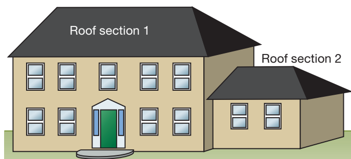
Figure 1: Example of residential building with two roof sections
